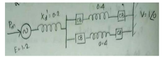
14. In the single machine is connected to infinite bus shown in below, the generator is delivering the real of 0.8 p.u at 0.8 p.f lagging to the infinite bus. The power angle of the generator in degrees is?14M
